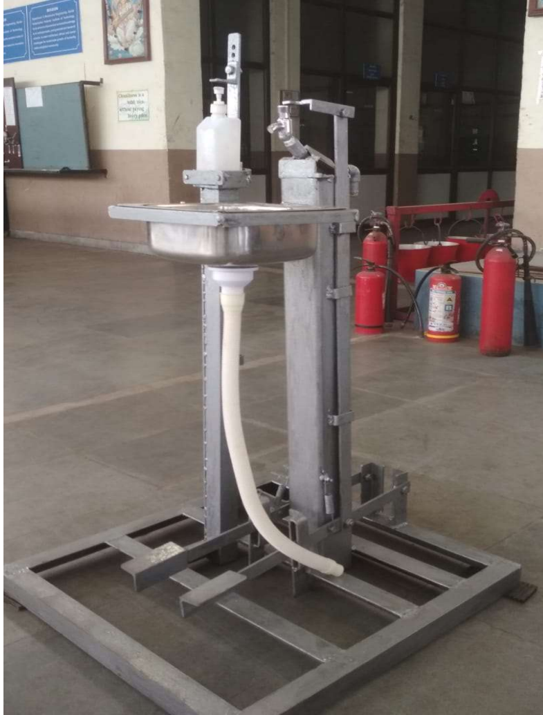
Foot Operated Sanitizer Dispenser Placed at the entrance to the Health Centre.
